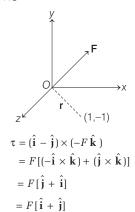
3 Torque due to central force is zero,
