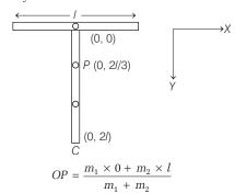
where,  $m_1$  and  $m_2$  are masses of horizontal and vertical section of the object. Assuming object is uniform,
